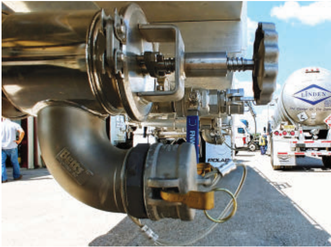
One of Linden's newest trailers is a custom Polar Tank Trailer with a Betts package of quick-clean valves and Vapor-Pro vapor recovery. Photo Jason McDaniel/BT
