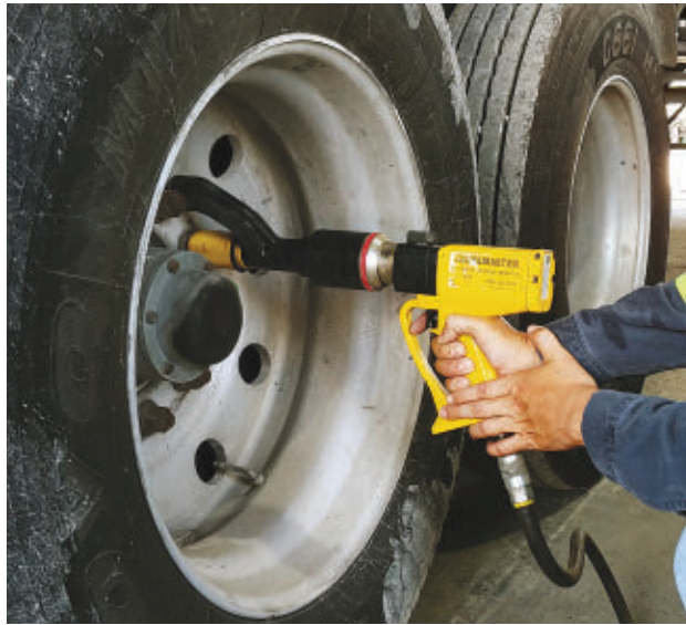
SmartWay-verified Michelin X One wide-base tires, at left, are designed to improve a fleet's bottom line. A Wheelmaster pneumatic torque wrench ensures wheel nuts are safely tightened to manufacturer specifications. Photos Jason McDaniel/BT
