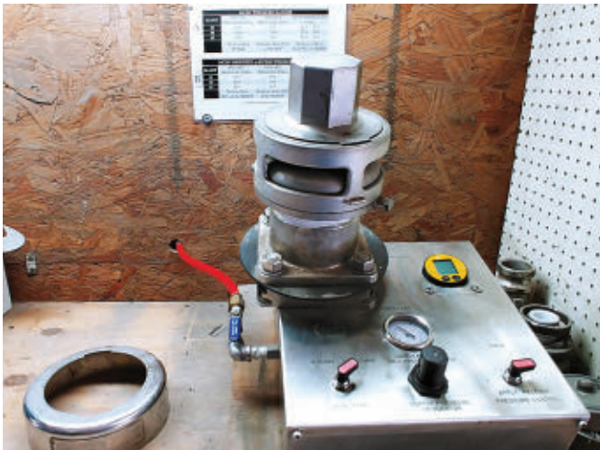
A Pelican Worldwide pressure/vacuum tester ensures Linden's trailer vents are up to code during HM-183 cargo tank inspections. Photo Jason McDaniel/BT
