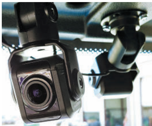
Linden Bulk, an Odyssey Logistics subsidiary, first deployed a dual-camera SmartDrive safety system, with inward- and front-facing cameras, in 2018.
