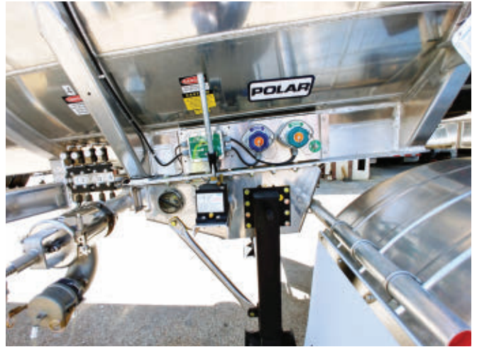
The 2021 Polar trailer, designed and spec'd out for a key customer, also boasts a Scully Load Anywhere Overfill Prevention System. Photo Jason McDaniel/BT
