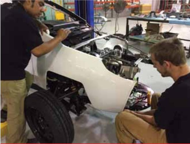
Technicians install the right-front fender of the Elio E-Series vehicle at the Elio Motors Pilot Operations Center in Livonia, Michigan. Elio Motors plans to build 23 E-Series vehicles for crash and validation testing, prior to moving to commercial production of the vehicle in its assembly facility in Shreveport, Louisiana. Image courtesy of Elio Motors.
